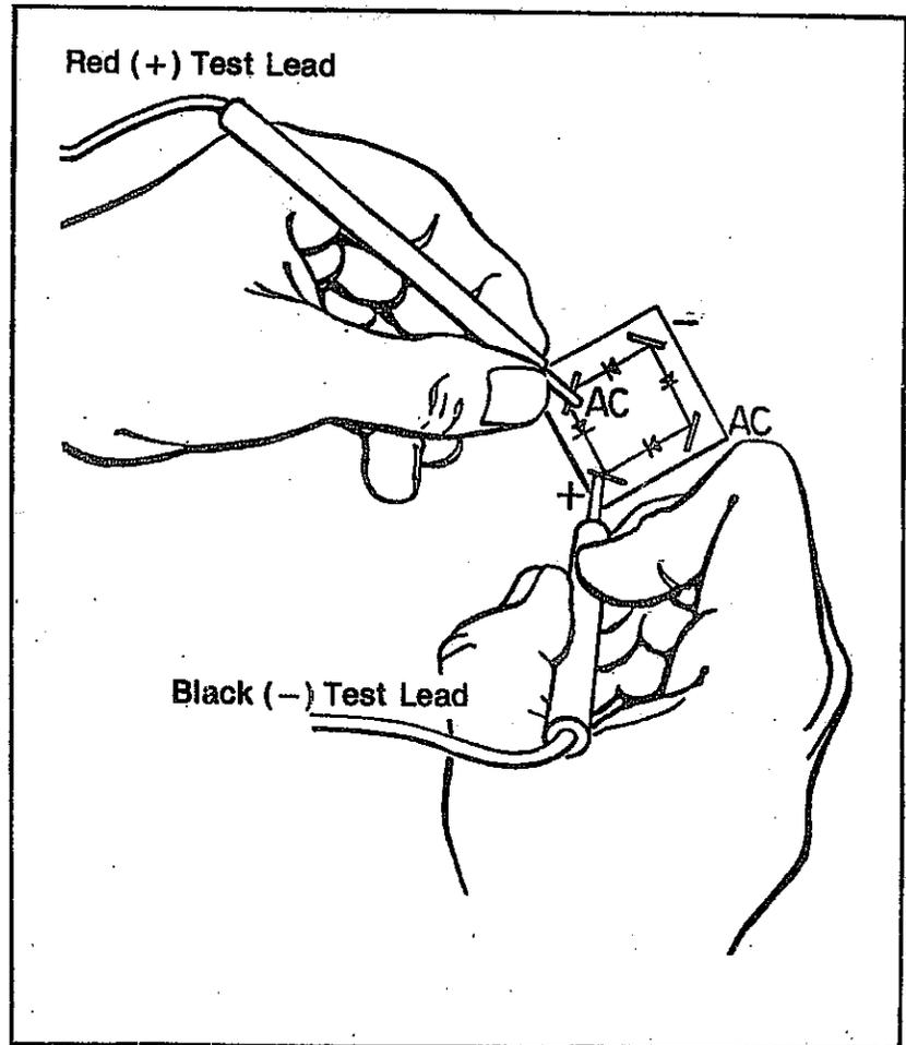
4. Check field coil resistance as per specification given in A-6.
